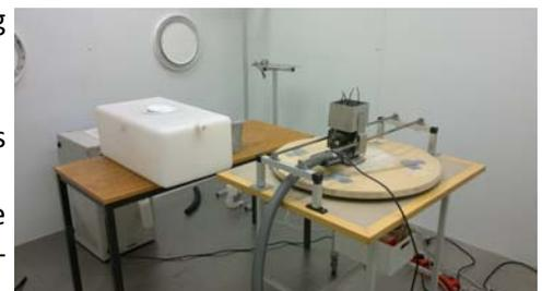
**Figure 2:** Equipment used for generation of sanding dust at NRCWE.
