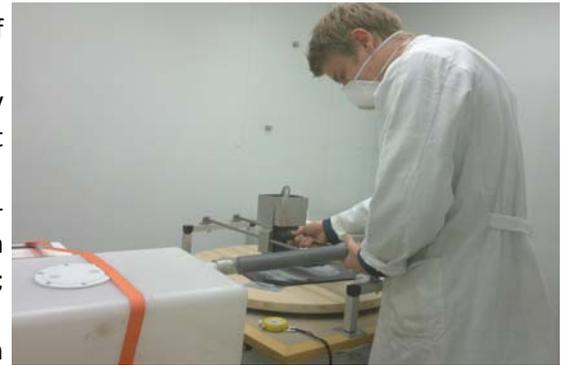
**Figure 2:** NRCWE scientist conducting sanding experiments.
